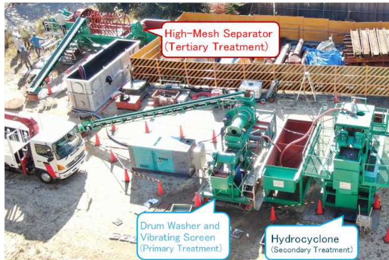
Figure 7-1: General View of the Sediment Classification Experimental Plant at Yahagi Dam (FY2023)
